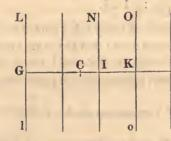
Let C be the place of the body, and take C K = C G; the part of the solid between G and K will have no effect on the body C, and therefore it is attracted to remain as if it were placed without it at the distance C K.
